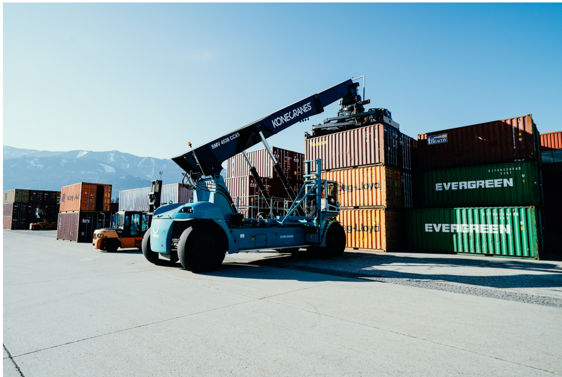
Figure 18: Diesel based reach stackers as currently used at LCAS (Image by ÖBB/Martin Hofmann)
